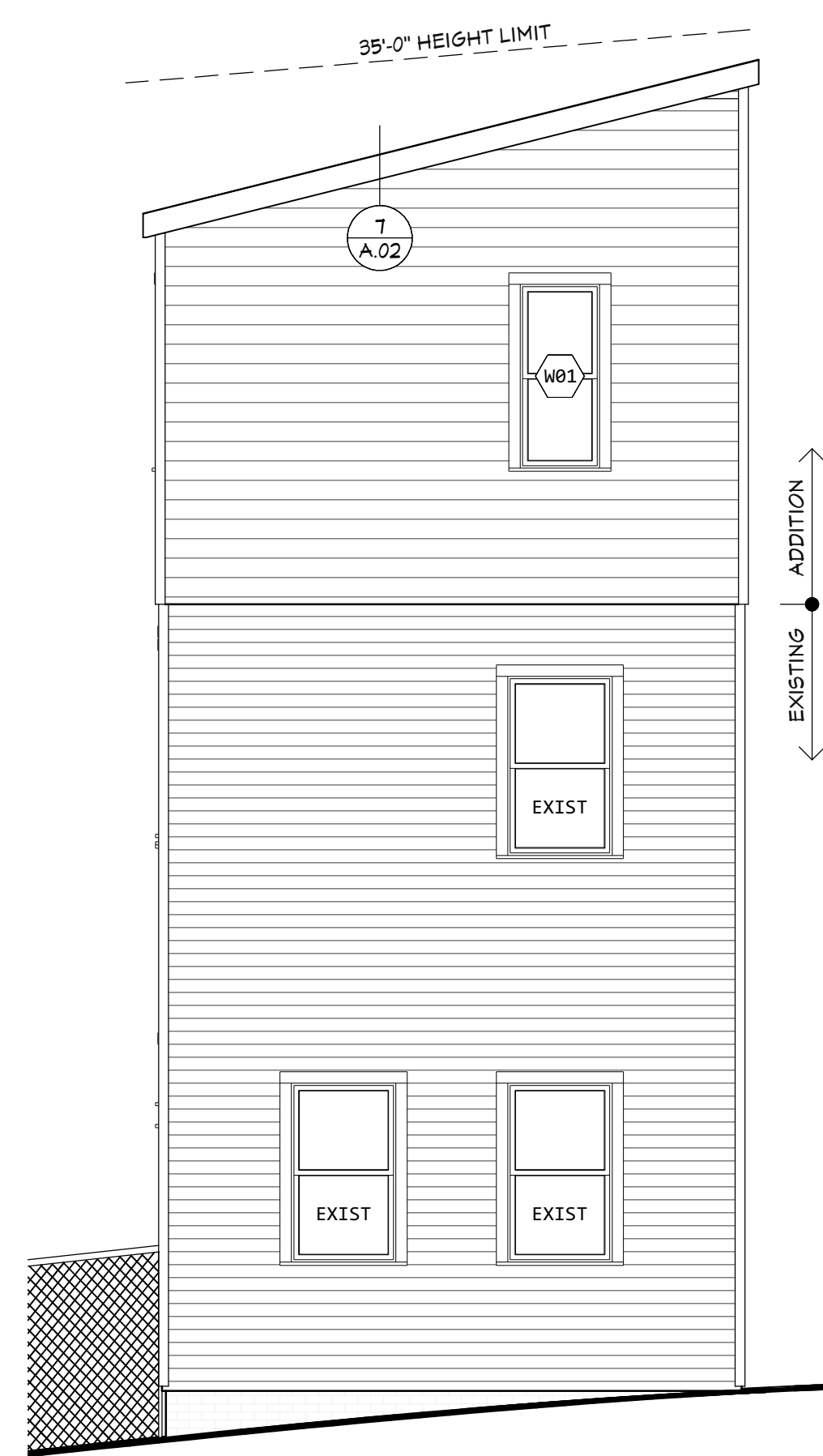
South Elevation : 1/4 in = 1 ft
